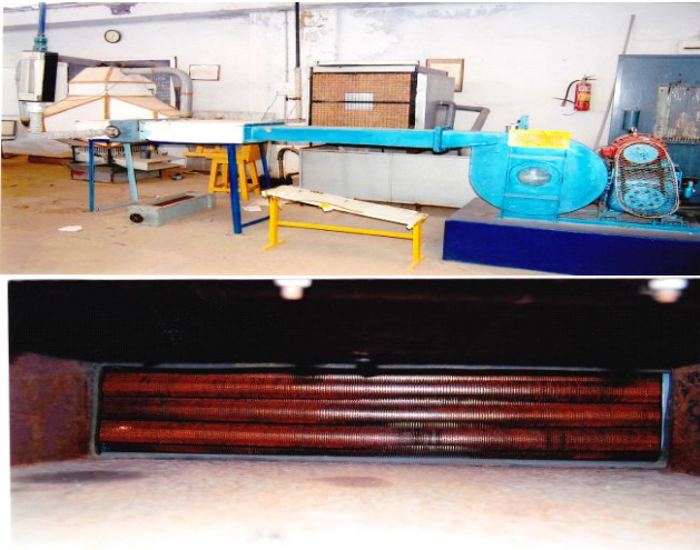
Fig.1. Photograph of experimental setup and cross flow multi tube heat exchanger
